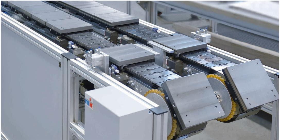
SPU 2040, dual-line, 114 chain width with positioning unit
