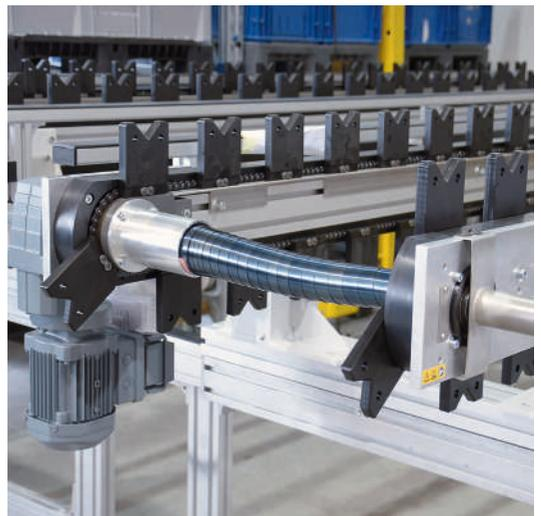
TKU 2040 for transporting camshafts with a spiraled cover as a protective guard on the connecting shaft
