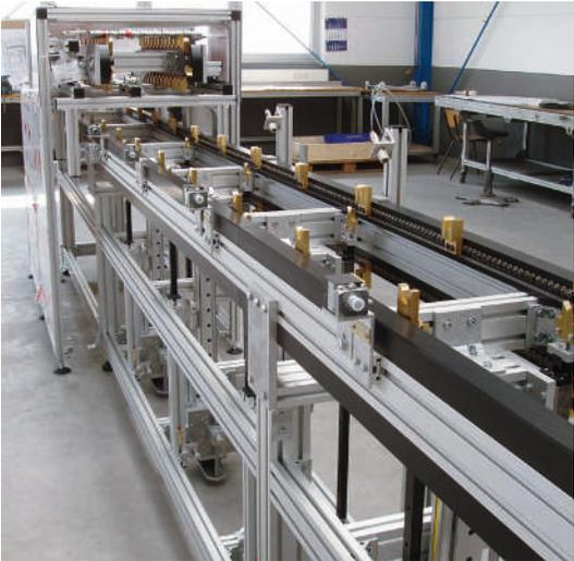
TKU 2040 with extractor unit and conveyor for rejected pieces
