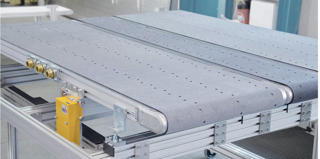
Multiple-line vacuum belt conveyor GUF- P2041 BC with electronically coupled drives
