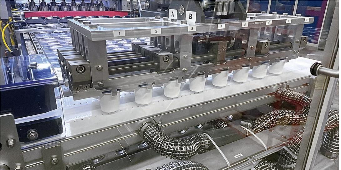
Vacuum belt conveyor GUF-P 2000 AC in the packaging industry, cycles at high accelerations without containers slipping or tipping over
