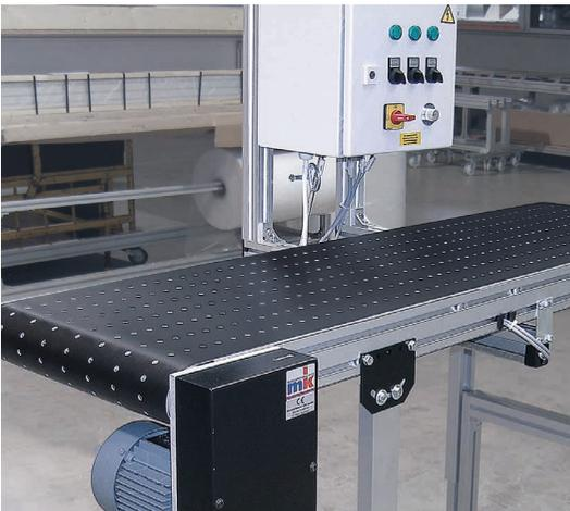
Vacuum belt conveyor GUF-P 2041 AC including frame and control unit
